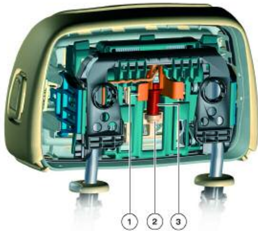
Pyrotechnic actuator (normal state)
